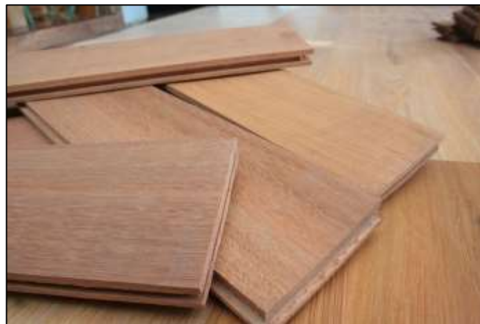
Figure 12: Wooden flooring made of bengkirai
